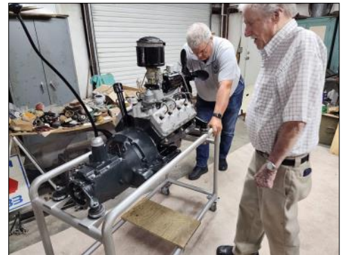
(Left and center) 1939 Ford V8 60 HP engine; (Right) Danny and Lawson Cox inspecting the engine.
