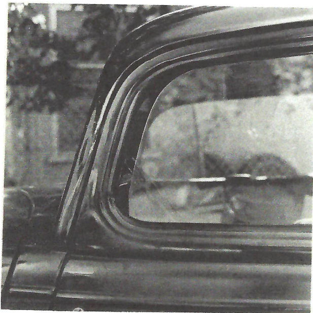
On '34s the front windows were built in such a fashion that they created a vent window when the crank was given an extra turn.
