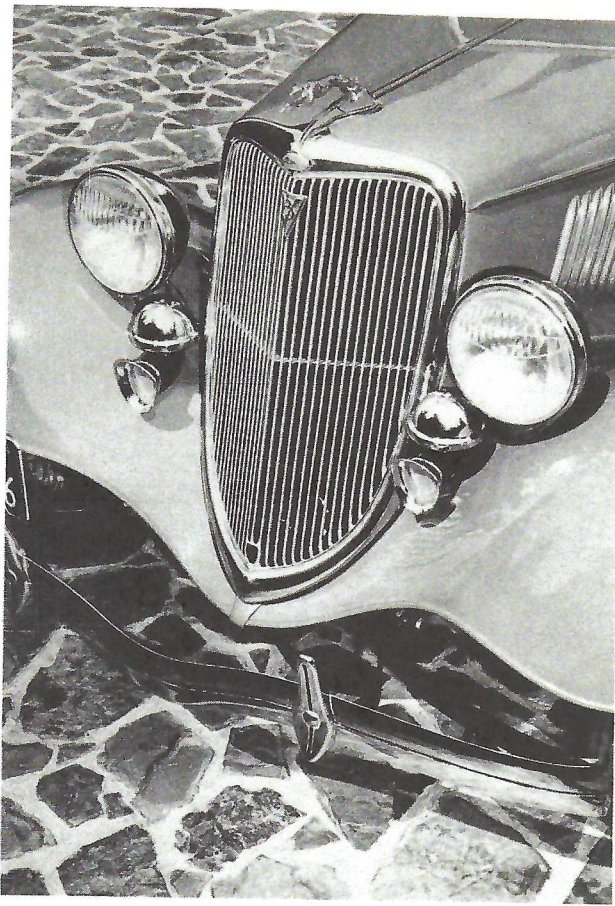
Front view of a '34 gives good look at the items peculiar to a '34. Note the V-8 emblem on the grille since it is much different than a '33. Bumper guards on this Ford are Ford-factory items.
