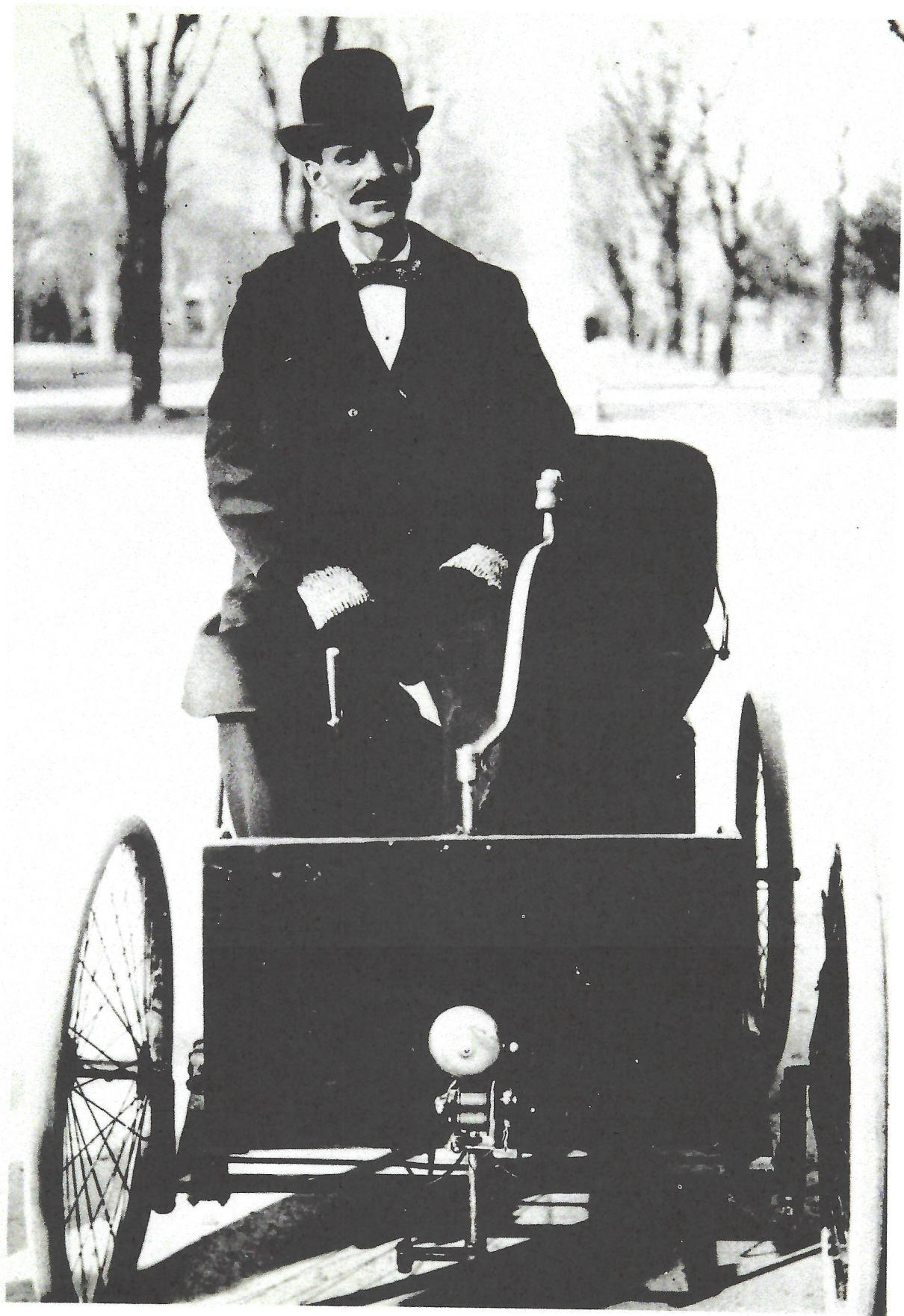
FIRST "BETTER IDEA" – Automotive pioneer Henry Ford was photographed in Detroit in his Quadricycle shortly after the initial pioneer run of his vehicle on June 4th, 1896. Although Ford Motor Company was founded in 1903, the birth of the multi-national corporation can be traced to completion of the Quadricycle 75 years ago. Mr. Ford's horseless carriage, powered by a two-cylinder, four-cycle engine, had a trolley-like electric bell to warn pedestrians.
