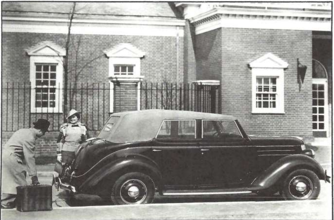
Early 1936 Convertible Sedan (left) had no trunk like the Phaeton. But later in the year Ford introduced the Convertible Touring Sedan which had a beautiful and functional trunk which was hinged at the top and housed the spare wheel with plenty of room left for luggage, etc. Interesting sidelight: Still no whitewall tires on this top of the line DeLuxe Ford! Ford Archives photo.
